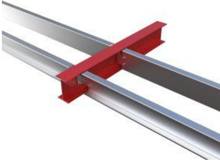
Figure 23. Indicative Steel Frame & Joist Inset System
